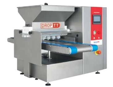
The DROP TT is a table top depositor for fast and efficient depositing of semi-liquid and more solid products. Keywords of this table top bakery machine are: compact, simple, fast and accurate.
