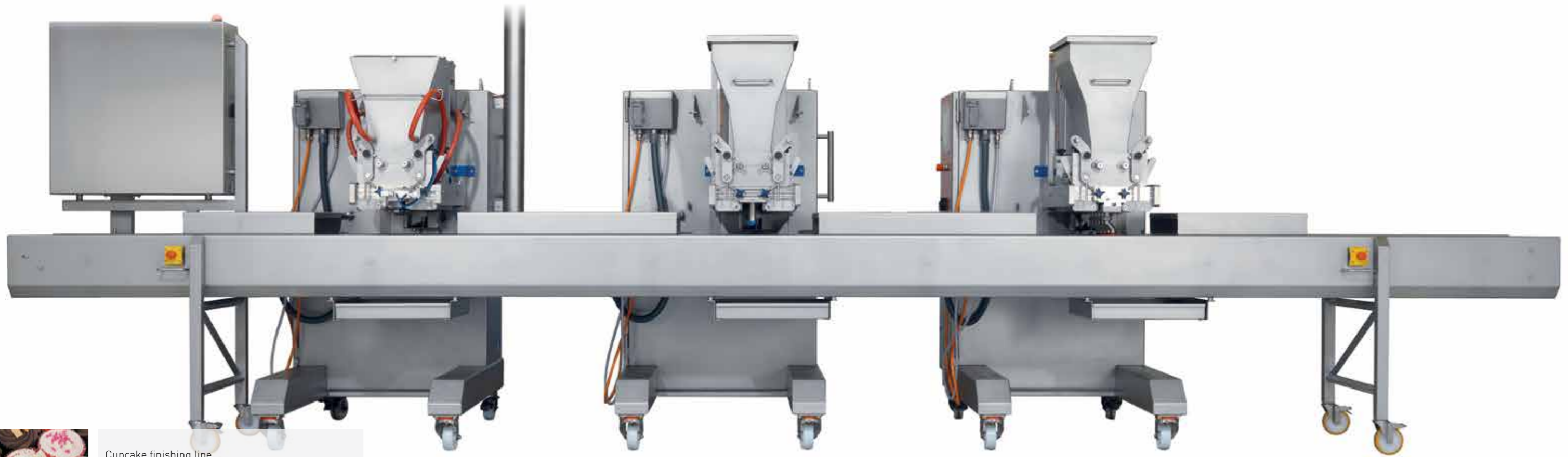
Cupcake finishing line injecting → ring decorating → star decoration
